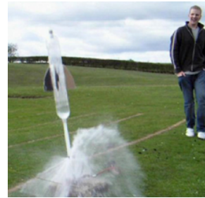
Figure 3.2: Water Bottle Rocket as an example of the principle of a launch vehicle applying Newton's third law. 4
