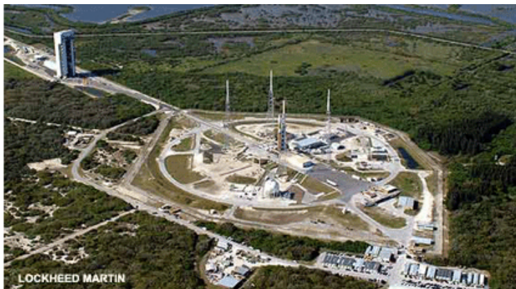
Figure 14.10: Launch Complex 41 at Kennedy Space Center, with an Atlas-V poised for launch amid four lightning rod towers (LC-41 was previously the launch pad for the Viking & Voyager missions). Image courtesy NASA.
