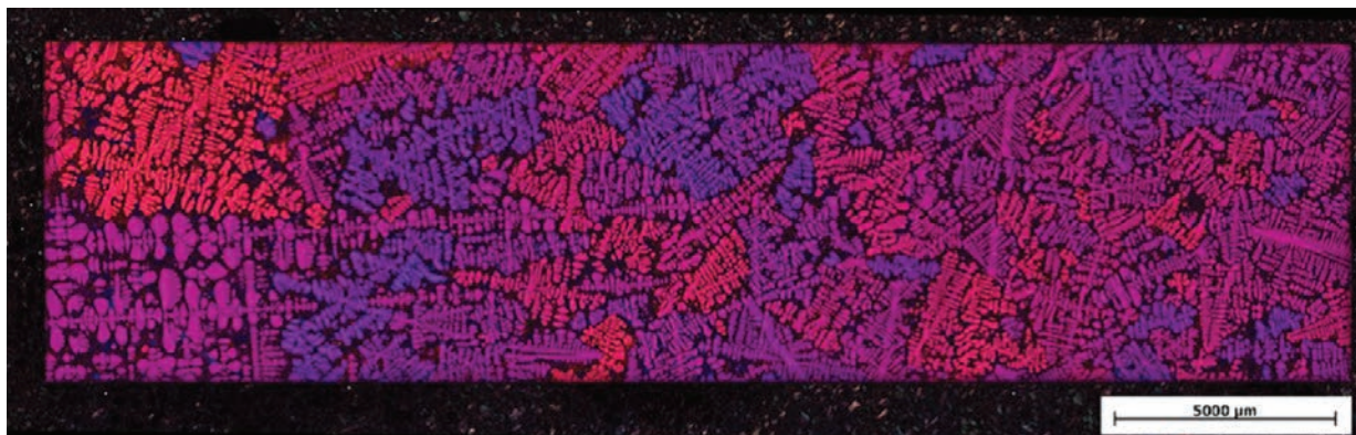
A typical microstructure obtained in a CETSOL sample containing a grain refiner. The sample was directionally solidified in the ISS Materials Science Laboratory.
