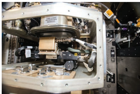
The Light Microscopy Module is configured for ACE-T-1 experiment.
