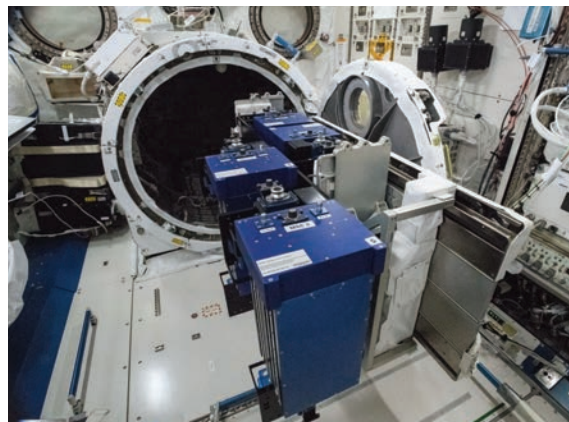
The Materials ISS Experiment-Flight Facility (MISSE-FF) in the Japanese Experiment Module (JEM) prior to transit through the JEM airlock inner hatch and mounting on the JEM external facility.
