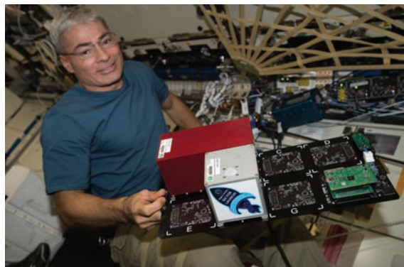
Flight Engineer Mark Vande Hei swaps out a payload card from the TangoLab-1 facility and places it into the TangoLab-2 facility. TangoLab provides a standardized platform and open architecture for experimental modules called CubeLabs. Pictured here are a pair of CubeLabs that are 2U and 1U in size.
