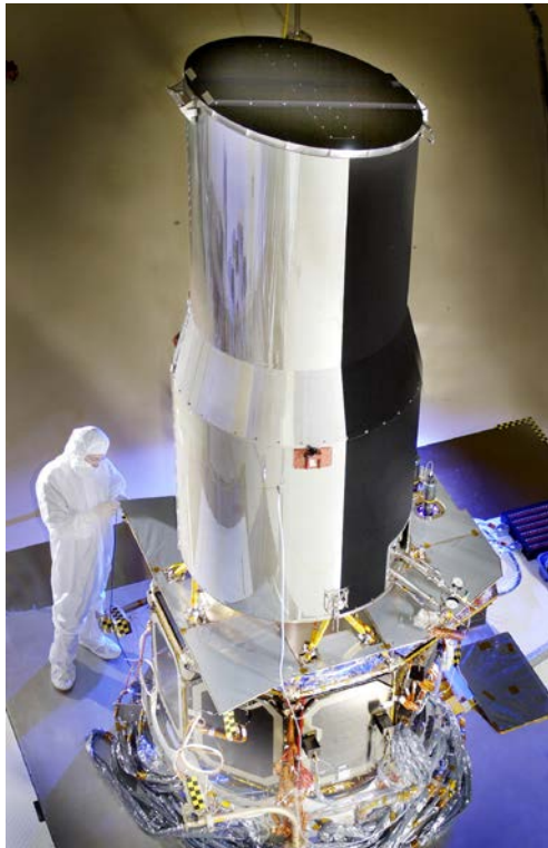
Image showing assembly of the Spitzer Space Telescope, the infrared telescope designed to study the early universe, young galaxies, and star formation. Credit: Russ Underwood, Lockheed Martin Space Systems; courtesy NASA/JPL-Caltech.
