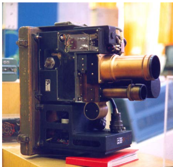
The Yenisey "photo-television unit" on board Luna 3 was developed by the Leningrad-based VNII-380 institute. It included a dual-objective camera (AFA-Ye1) developed by the Krasnogorsk Mechanical Plant. The camera took two pictures simultaneously using a 200 mm lens and a 500 mm lens. Credit: T. Varfolomeyev
