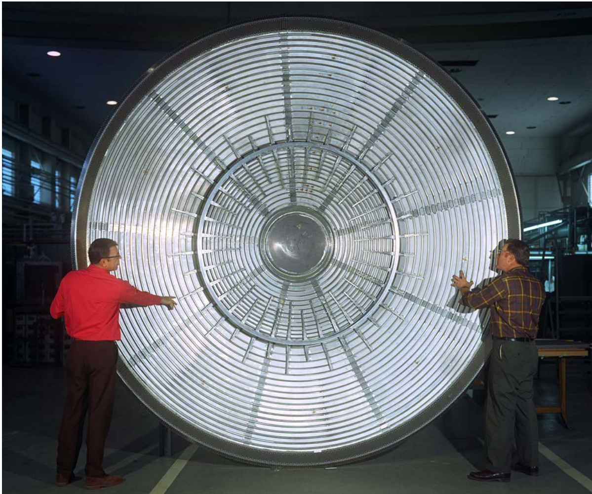
NASA scientists at the Langley Research Center in Virginia stand in front of the aeroshell that protected the Viking Lander 1 during its entry into the Martian atmosphere in 1976. The aeroshell was made of the heat shield and a “back-shell” which contained parachutes and other components used for entry. Credit: NASA/JPL
