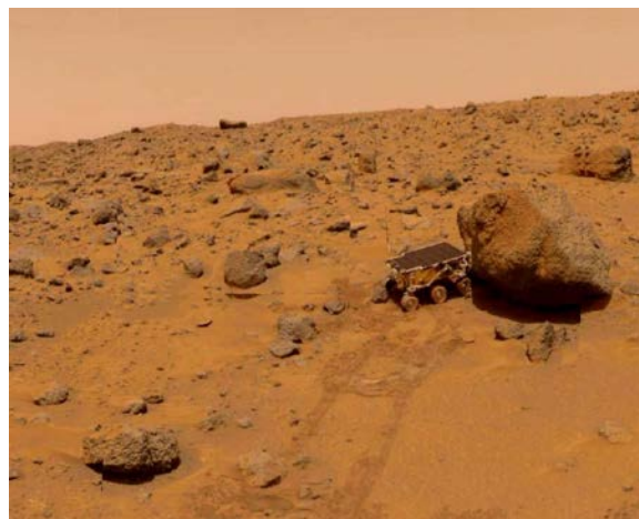
On 21 July 1997, the Mars Pathfinder's Sojourner rover takes its Alpha Particle X-ray Spectrometer measurement on a rock near the landing site. Credit: NASA/JPL
