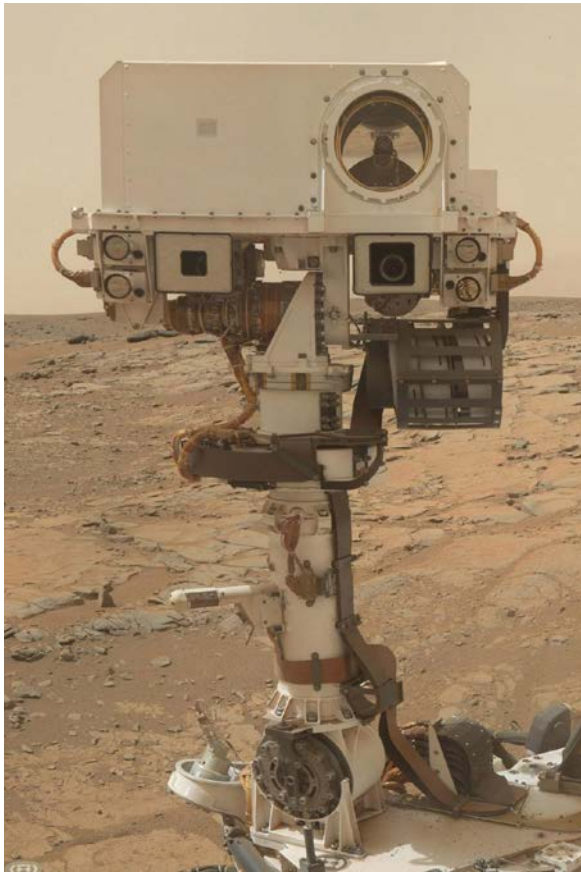
Visible at the bottom (the thick vertical rod) is the Rover Environmental Monitoring Station (REMS) built by the Centro de Astrobiología (CAB) in Madrid, Spain. The pencil-like instrument sticking out to the left is Boom 1 which houses a suite of infrared sensors to measure the intensity of infrared radiation emitted by the ground. The large structure at the top includes the Mastcam (Mast Camera) and the white rectangular-shaped ChemCam (Chemistry & Camera) instruments. Credit: NASA/JPL/MSSS/Ed Truham
