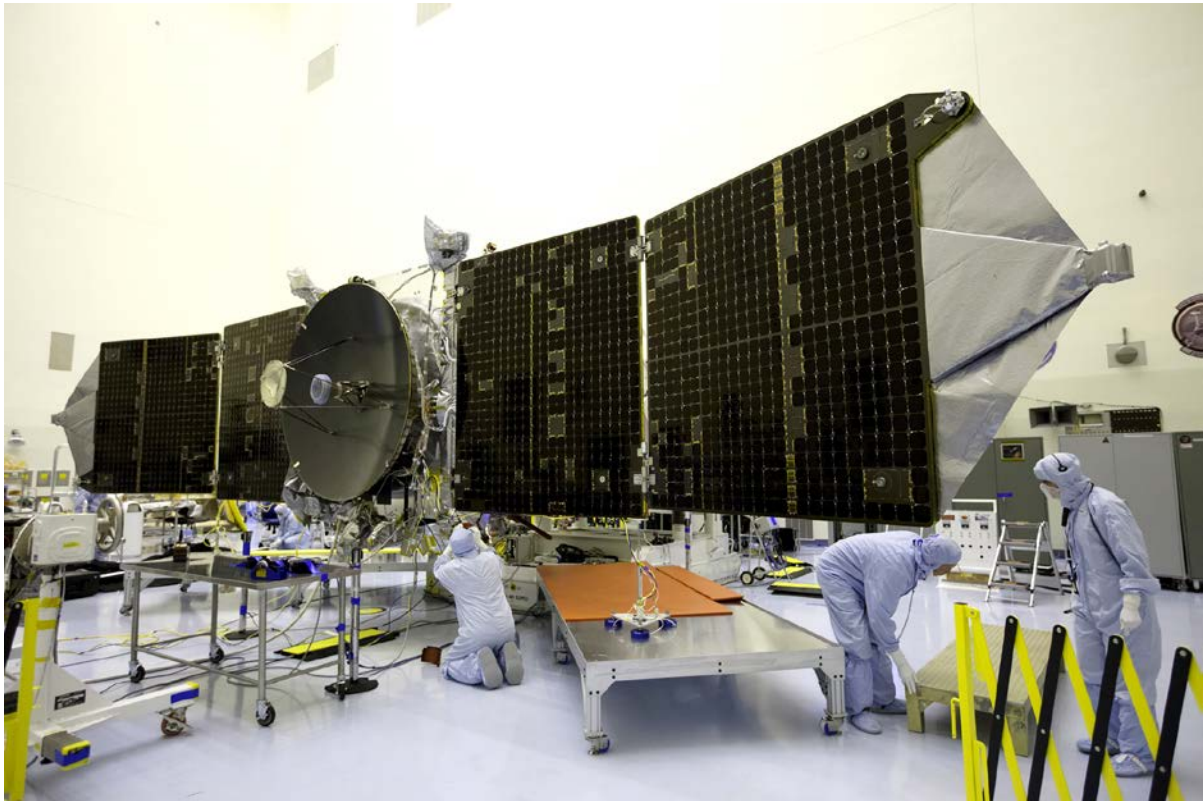
Engineers and technicians test deploy the two solar panels on NASA's MAVEN spacecraft. The image was taken in the Payload Hazardous Servicing Facility at NASA's Kennedy Space Center before launch in November 2013. Credit: NASA/Kim Shiflett
