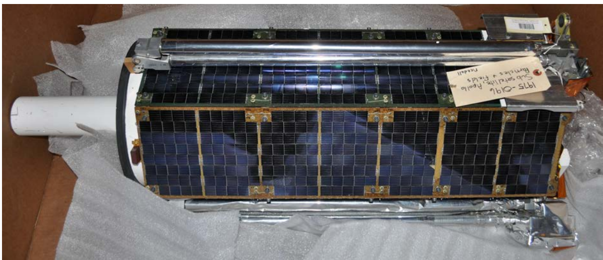
A ground model of the Apollo 15 Particles and Fields Satellite. Credit: NASA
