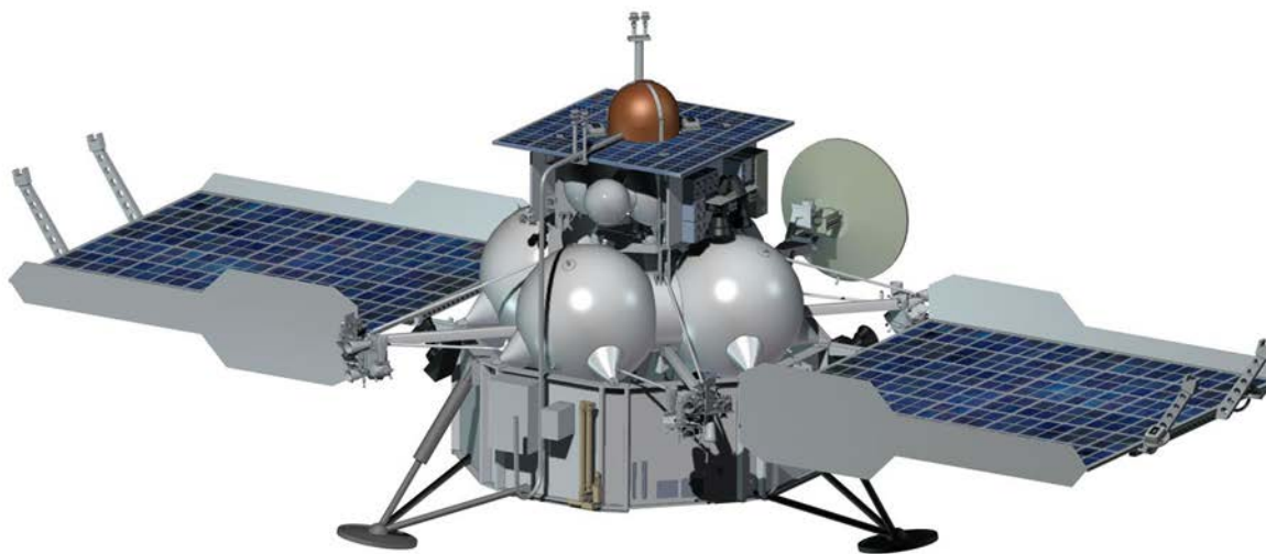
A simplified illustration of the Russian Fobos-Grunt lander package. The half-spherical object at the top was the descent capsule that would carry samples from the Martian moon Phobos back to Earth. Credit: ESA/Lavochkin Association
