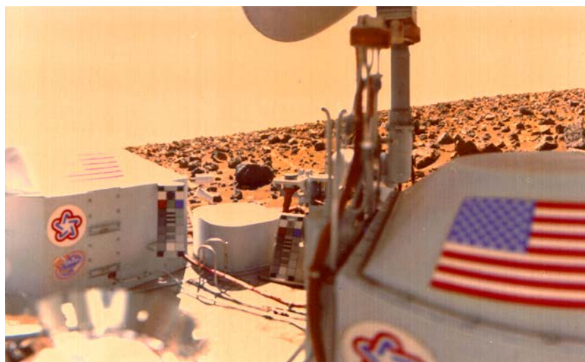
Viking 2 Lander image showing the spacecraft and part of Utopia Planitia, looking due south. The American flag, color grid, and bicentennial symbols (for the 200th anniversary of the Declaration of the Independence, celebrated in 1976) are visible in this image, and were used to calibrate color images as they were received on Earth. The image was taken on 2 November 1976. Credit: NASA/JPL
