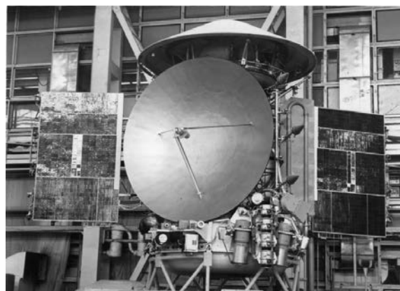
The Soviet Mars 6 spacecraft. The lander aeroshell is visible on top. Credit: Don Mitchell
