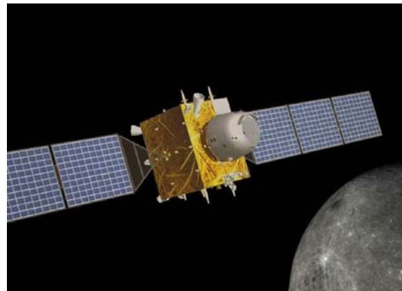
Artist's rendering of the Chinese Chang'e 5-T1 spacecraft. The headlight-shaped object is the descent module that was successfully recovered after its circumlunar mission. Credit: chinaspacereport.com
