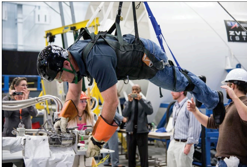
Figure 8. Astronaut Doug Wheelock is testing fluid QDs at varying line pressures to determine which pressures make it too hard for the spacewalking crew to perform the task. Doug had performed a similar task while on a spacewalk in 2010, so he was the natural choice to perform the testing. A harness allowed his body to move left and right when he put in forces on the connectors, somewhat simulating the way it would be in space.
