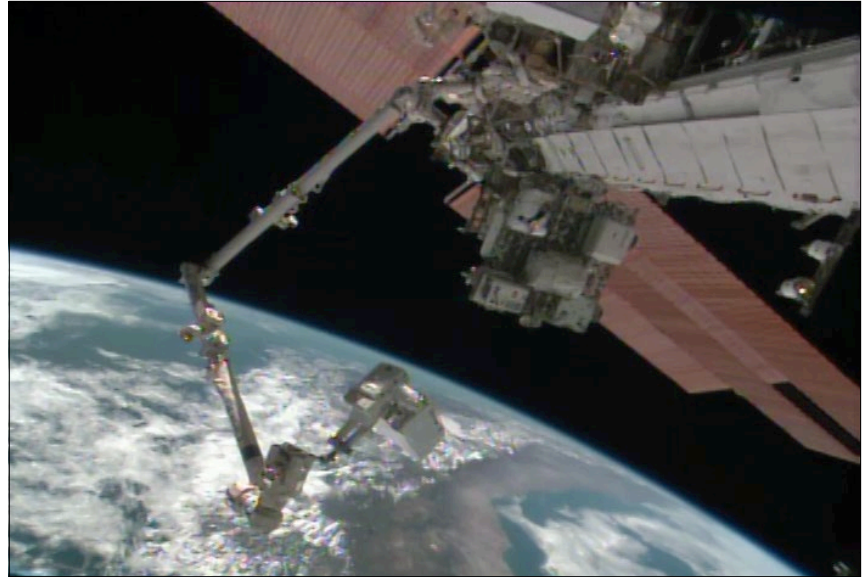
Figure 14. Astronaut Mike Hopkins rides the robotic carrying the 354-kg (780-lb) ammonia Pump Module as the ISS flies over South America.
