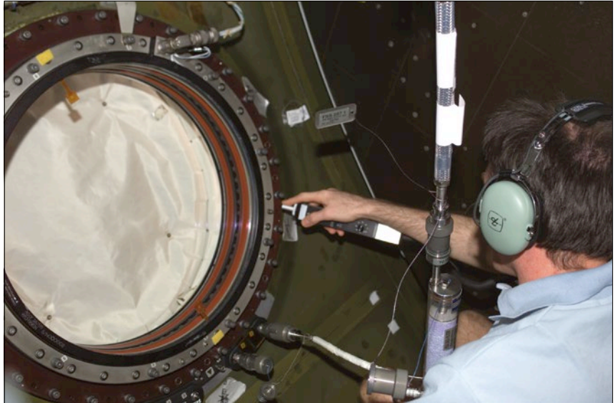
Figure 19. Expedition 8 Commander Mike Foale using the Ultrasonic Leak Detector in 2004 to pinpoint a small leak that had developed in one of the seals of the hose used to maintain a vacuum between the panes of glass within the large window of the US Laboratory. Once the leak point was identified, the hose was disconnected (which stopped the leak to space) until a replacement hose could be flown to the space station.
