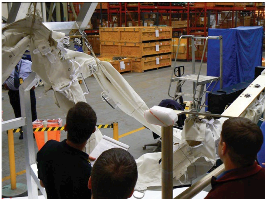
Figure 7. The spacewalking astronauts from STS-130/ISS-20A and EVA team try to figure out a new routing of the ammonia lines and the insulation using a crude mock-up of where the connectors would be on the various modules.
