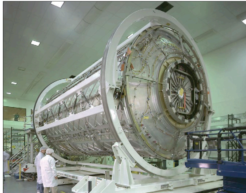
Figure 3. The US Laboratory module, Destiny, is supported by a frame that allows it to be rotated as it is being built. The reinforcing ribs that make up a waffle pattern that crisscrosses the primary pressure shell of the module can be seen. These pieces are normally under the orbital debris shielding and thermal insulation that makes each module appear smooth and round (as with Node 3 in Figure 2). This reinforcement is what gives each module enough strength to contain the atmospheric pressure that allows the crews to work in a shirtsleeve environment.
