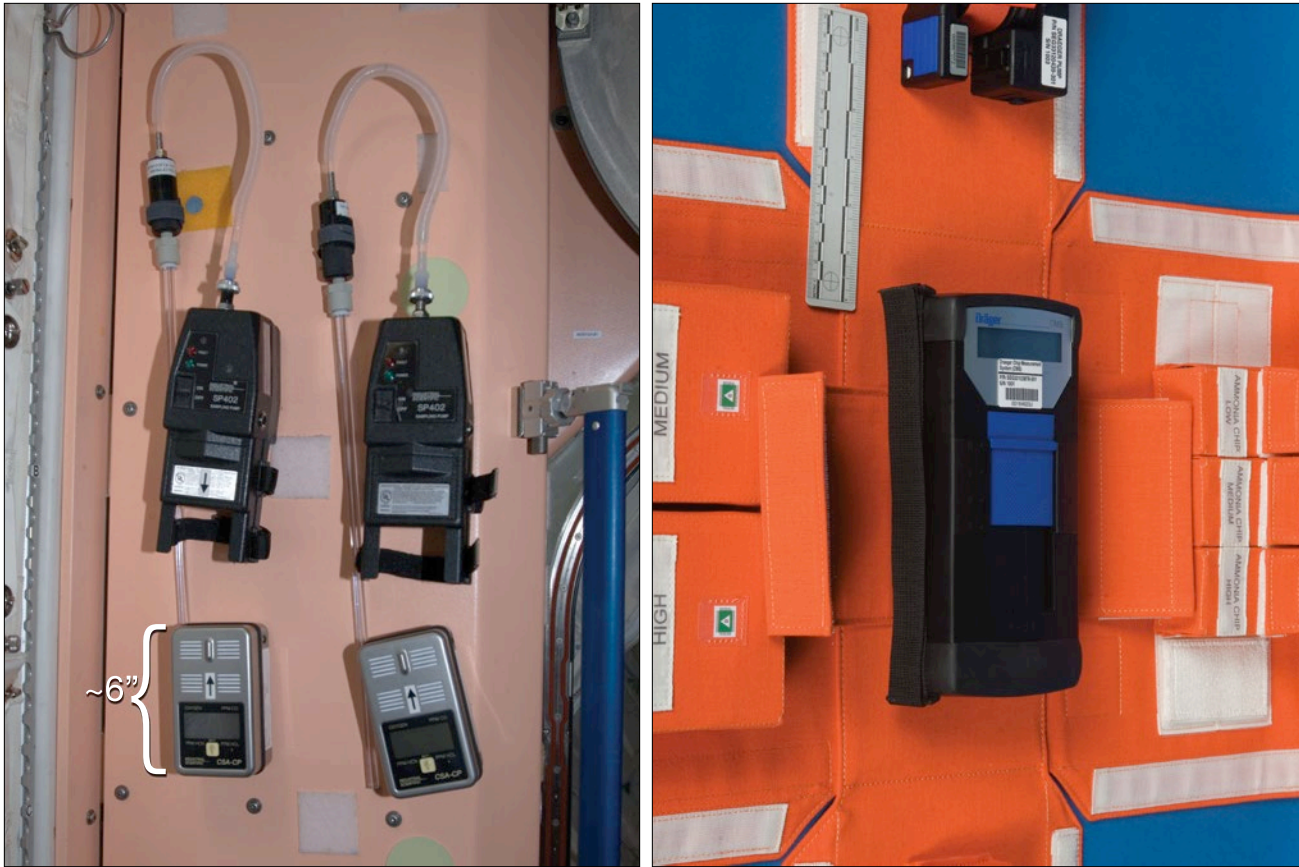
Figure 2. GSA-CP (left) attached to the wall of Node 1 and CMS (right). For the CSA-CP, the metal detector (gray), which is about 15 cm (6 in.) in length, is placed in the black holder that pumps air in through a tube, which is currently connected to a long rod that can be inserted into racks.
