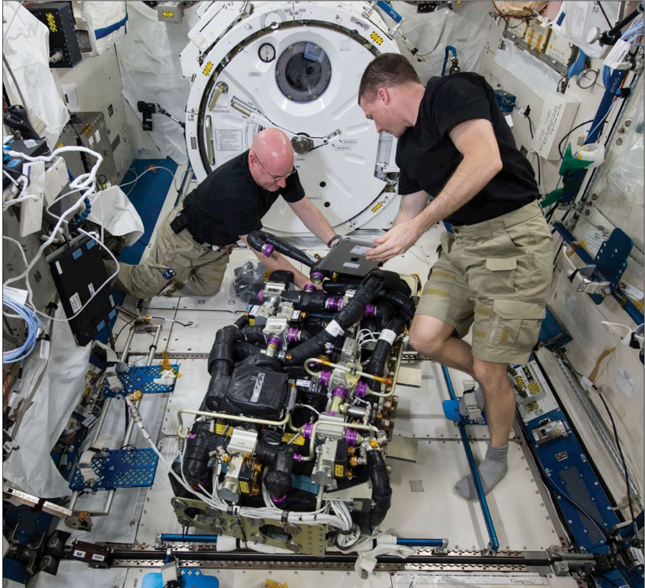
Expedition 43 astronauts Scott Kelly (left) and Terry Virts perform in-flight maintenance on the Carbon Dioxide Removal Assembly. The inner workings of the device were removed from the rack in Node 3 and moved to the Japanese Experiment Module to provide a larger area in which the crew can work.
