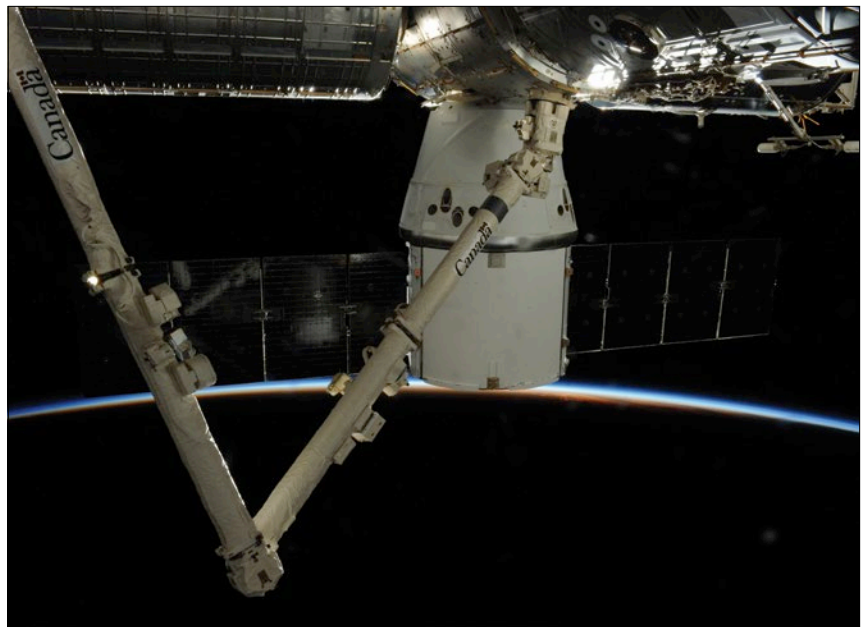
Figure 3. View of the berthed SpaceX Dragon Commercial Resupply Services-3 spacecraft on April 26, 2014, Canadarm2 SSRMS, and portions of the forward ISS in front of an orbital dawn.
