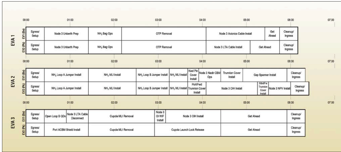
Figure 17. The final EVA timelines. EVA 1 consisted of preparing Node 3 for berthing. First the LTA power cable that powered the heaters was disconnected and bolts holding the module in the cargo bay were released. While the robotic arm was moving Node 3 from the orbiter cargo bay to its berthing spot, the crew performed other tasks such as positioning the bag that holds the ammonia hoses and removing the Orbital Replacement Unit Tool Platform. Once berthed, the spacewalking astronauts reconnected the heater cable as well as an avionics computer cable that would allow the computers to talk to the rest of the ISS systems. On EVA 2, the ammonia line of the “A” side of the cooling system was installed, and MLI (see Figure 14) was installed. This was repeated on the “B” side. The trunnions, which helped hold the module securely in the cargo bay, were then covered to prevent heat from leaking away from the module. During EVA 3, the Loop “B” cooling was fully integrated into the ISS system (Loops B QDs) followed by removal of the MLI that protected the Cupola and the releasing of locks that held the shutters in place during launch. The LTA heater cable, which was no longer needed since Node 3 systems were now fully functional, was removed. Other small tasks were performed on all three EVAs. The Get Ahead section on the last spacewalk consisted of a list of small tasks that were not required for STS-130/ISS-20A but that had to be performed at some point; time permitting, the EVA officer picked tasks from a list of various options for the crew to perform.
