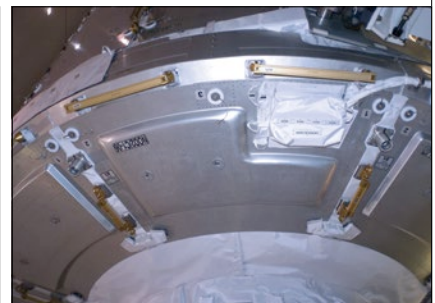
Once the MLI blankets are installed, the MMOD shields can be installed. Some equipment, such as these EVA handrails on Node 2, are also installed onto the outside of the shields. The shields are designed to be easily removable by spacewalking astronauts to access the equipment under the shields and MLI blankets.
