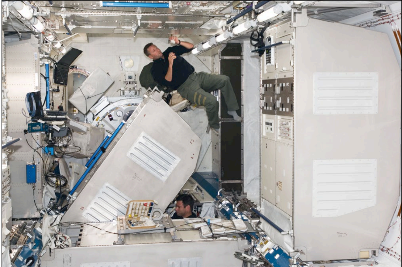
Figure 24. Astronauts Ken Ham (top), STS-124 pilot, and Greg Chamitoff, Expedition 17 flight engineer, install various racks in the JEM module after it was attached to the ISS on STS-124/ISS-1J (2008). Some of the racks were launched in one location due to orbiter center of gravity requirements and needed to be moved to their final locations after the module was attached to the ISS.
