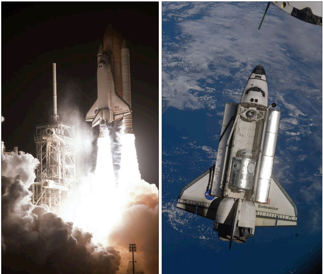
Figure 15. Launch of Space Shuttle Endeavour on February 8, 2010 (left). View of Endeavour's cargo bay from the ISS showing Node 3 with Cupola attached to the end. Due to the weight of the module, the rest of the cargo bay was empty.
