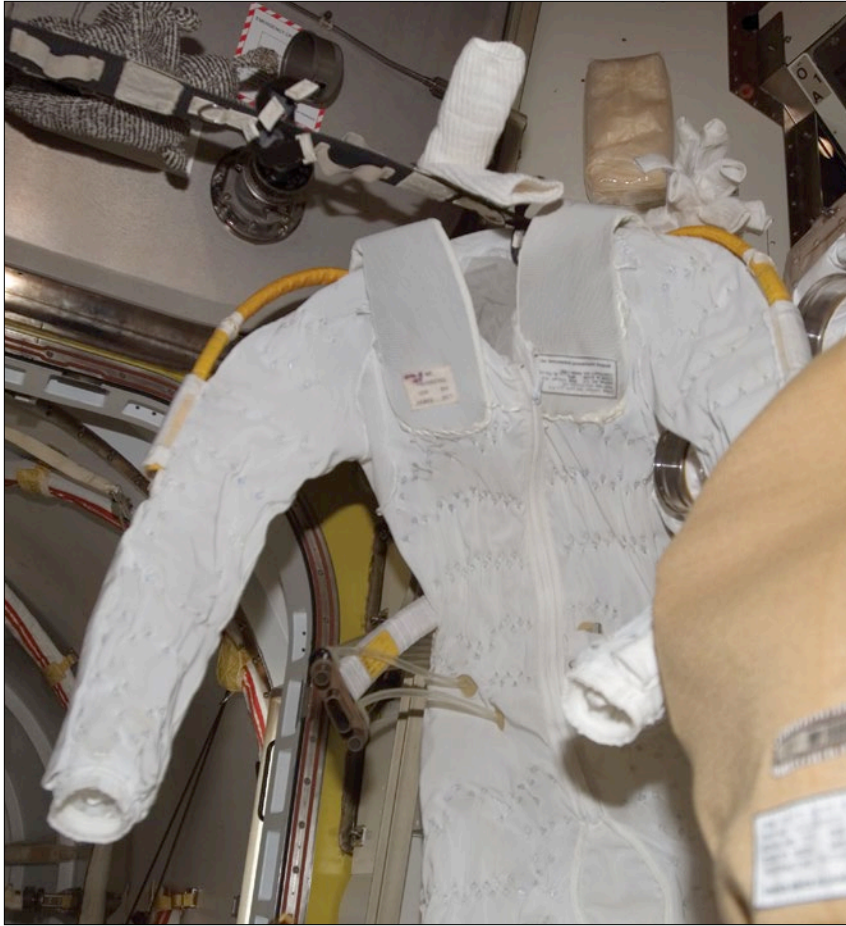
Figure 7. An LCVG, with its small water-filled tubes throughout and larger yellow ventilation ducts on the shoulders, floats in the airlock. The water tubes and ventilation ducting come together at the right waist with a connection point to the spacesuit. The fan/pump/water separator in the suit's backpack (not shown) provides the circulation. Shoulder pads provide a cushion from hard points in the suit and help fill some volume for an overall snug and comfortable fit.
