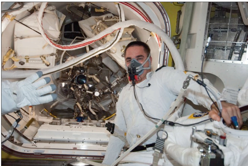
Figure 23. Astronaut Chris Cassidy is shown prior to an EVA during one portion of his prebreathe of pure oxygen to prevent DCS. In addition to an oxygen mask, he is wearing his LCVG, with small water-filled tubes throughout and larger ventilation ducts, as seen on his left arm and on his right waist. The Crewlock that goes to vacuum (located behind Cassidy) is filled with tools and storage bags. The suit umbilicals are attached to an umbilical interface panel in the Crewlock on one end and the EMUs on the other end. The EMUs are in the Equipment Lock in the foreground. One suit umbilical is routed under Cassidy's arm and is connected to a suit, seen in the lower right corner of the photo.
