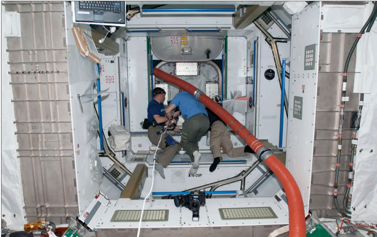
Figure 18. The 7-m (23-ft) long duct extended through Node 3 and into the Cupola to ensure proper airflow. Pictured are NASA astronauts Jeffrey Williams (center), Expedition 22 commander; Terry Virtz (left), STS-130 pilot; and Nicholas Patrick, STS-130 mission specialist.
