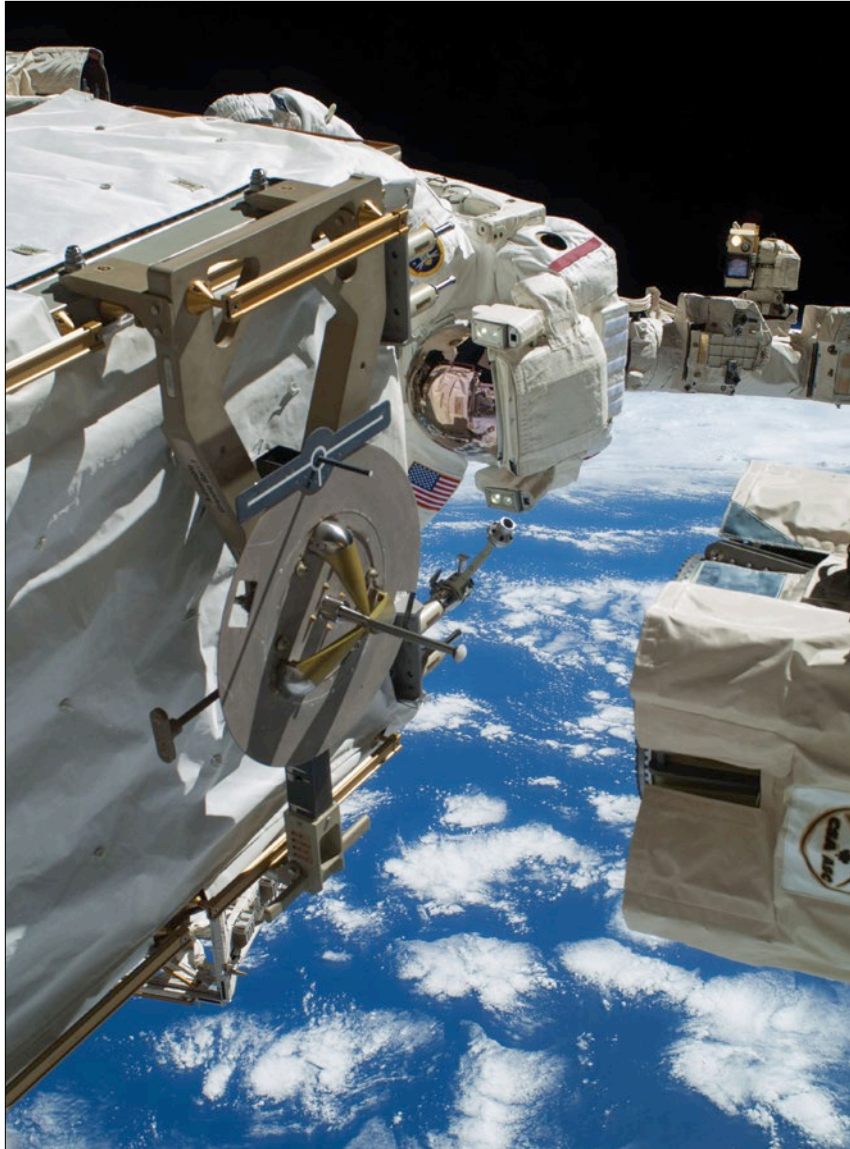
Figure 13. Expedition 38 Flight Engineer Rick Mastracchio, as seen behind part of the degraded Pump Module that was removed from the S1 truss during EVA 24. He is temporarily stowing the Pump Module by guiding it to be grasped by its grapple fixture by a robotic end effector that is housed on the Mobile Remote Servicer Base System.
