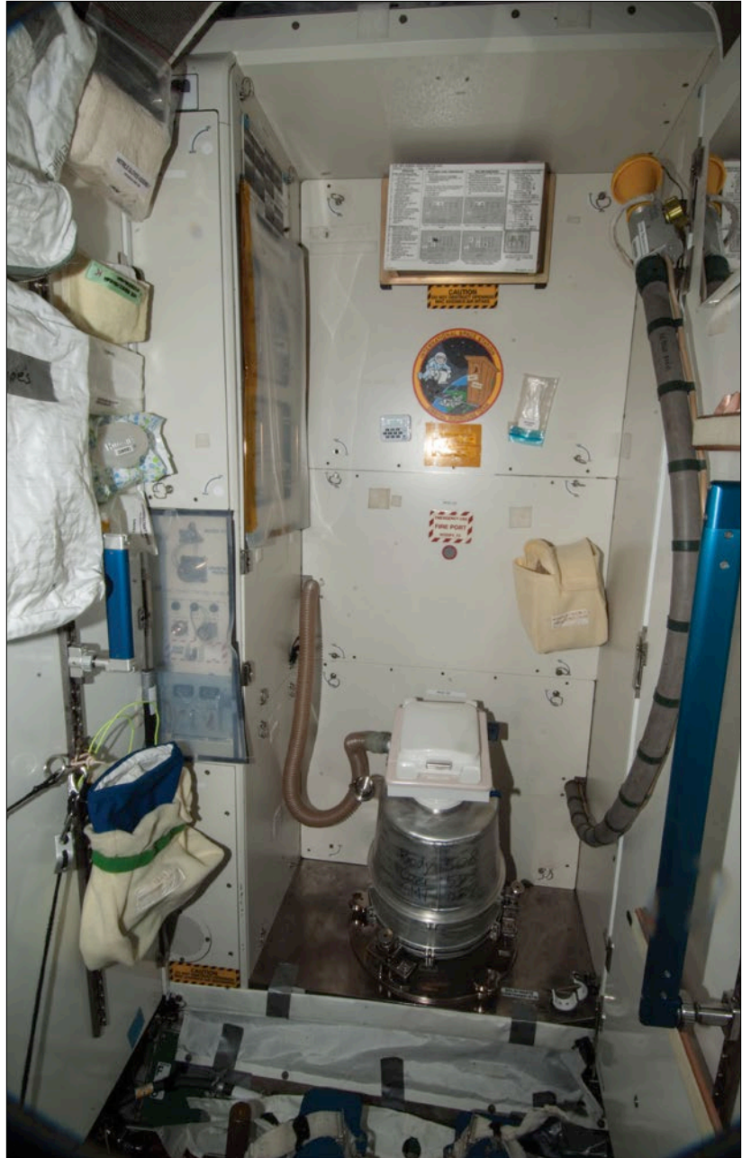
Figure 27. The Waste and Hygiene Compartment (WHC), located at NOD3F4, is an example of a rack designed for crew support. The WHC is the bathroom for the US Segment. To use this facility, crew members close a privacy curtain (located approximately where the camera was located to take this photo). Liquid waste enters a funnel at the end of the hose, as seen in the upper-right corner of the above image. Solid waste goes into the solid waste receptacle (metal can), as seen in the middle of the image. Liquids and solids are drawn into their respective destinations by airflow from a fan that runs when the WHC is powered on.
