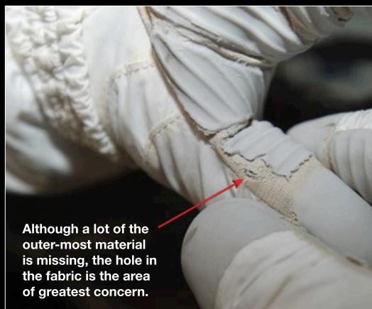
Figure 6. Glove tears that were noted during an EVA on STS-118/ISS 13A.1, causing the flight control team to terminate the EVA (i.e., bring the crew member back into the airlock early) as a preventative measure. Fortunately, the bladder that holds in the oxygen and keeps pressure on the astronaut was not damaged. Only the outer layers and fabric were affected.
