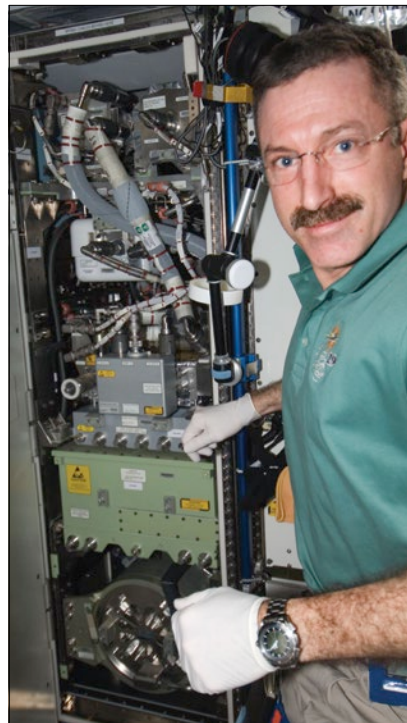
Figure 1. Astronaut Dan Burbank works on the OGA during Expedition 30.
