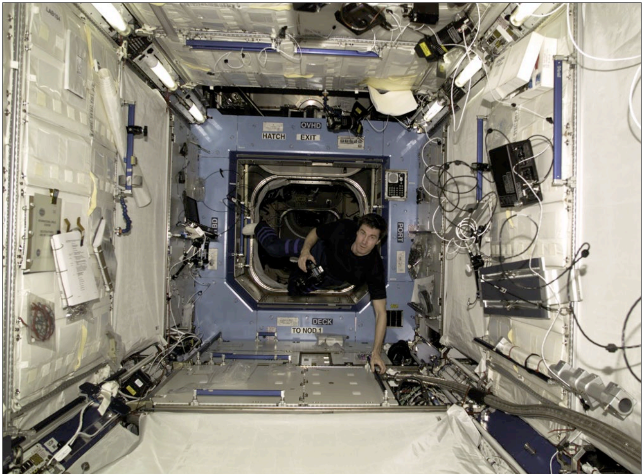
Figure 22. Cosmonaut Sergei Krikalev, flight engineer for the Expedition 1 crew, floats in the US Laboratory shortly after it was installed on STS-98/ISS-5A (2000). The four walls are actually the front faces of different racks. Note the empty central corridor. This photo was taken before the numerous science racks were launched and installed in the Laboratory.
