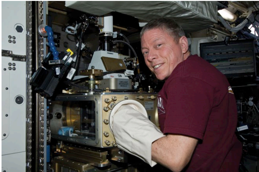
Figure 28. The Fluids Integrated Rack (FIR) at LAB1S4 is an example of a payload facility rack. Here, Expedition 29 Commander Mike Fossum works on an experiment inside the glove box that is part of the FIR rack (2011).
