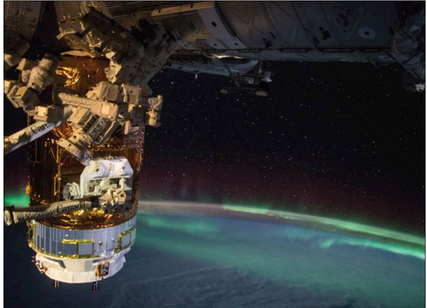
Figure 2. The Japan Aerospace Exploration Agency Kounotori HTV-5 is seen berthed to the ISS (vertical, left side of image). The external CALometric Electron Telescope experiment, which will search for signatures of dark matter, is seen being extracted from the unpressurized section by the station's robotic arm, Canadarm2. An aurora over the Earth limb is visible in the background. Photo is from August 25, 2015.
