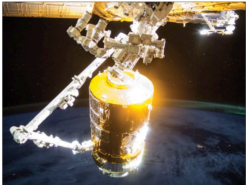
Figure 16. The HTV5 being maneuvered toward the Node 2 nadir Common Berthing Mechanism on the ISS (top of image).
