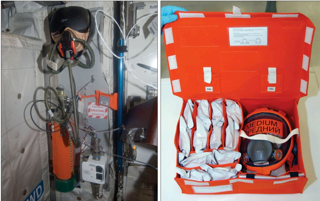
Figure 12. PBA (left) and respirator with fire cartridges (right). Different filters (orange boxes on either side) are attached to the respirator when it is being used after a fire or a toxic spill release such as ammonia.
