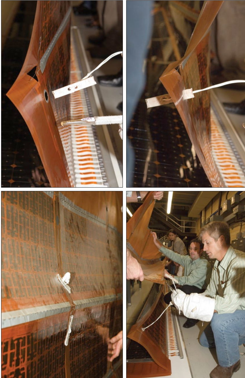
Figure 14. Repair technique development during STS-120/ISS-10A. Hinge stabilizing wires were called cufflinks because the crew would insert a thin 10 cm (4 in.) long aluminum plate through a hole, where it would catch on the other side. This plate was attached via a long wire to another plate that the crew would also thread through the array and into a hole on the other side of the damaged hinge. The first two figures show the insertion technique. The third photo shows the backside, where the wire is not visible but the aluminum plates are seen flat against the array. In the last photo, astronaut Steve Swanson tries out the technique while wearing an EVA glove to test whether Parazynski will be able to perform the technique while suited in the Extravehicular Mobility Unit.
