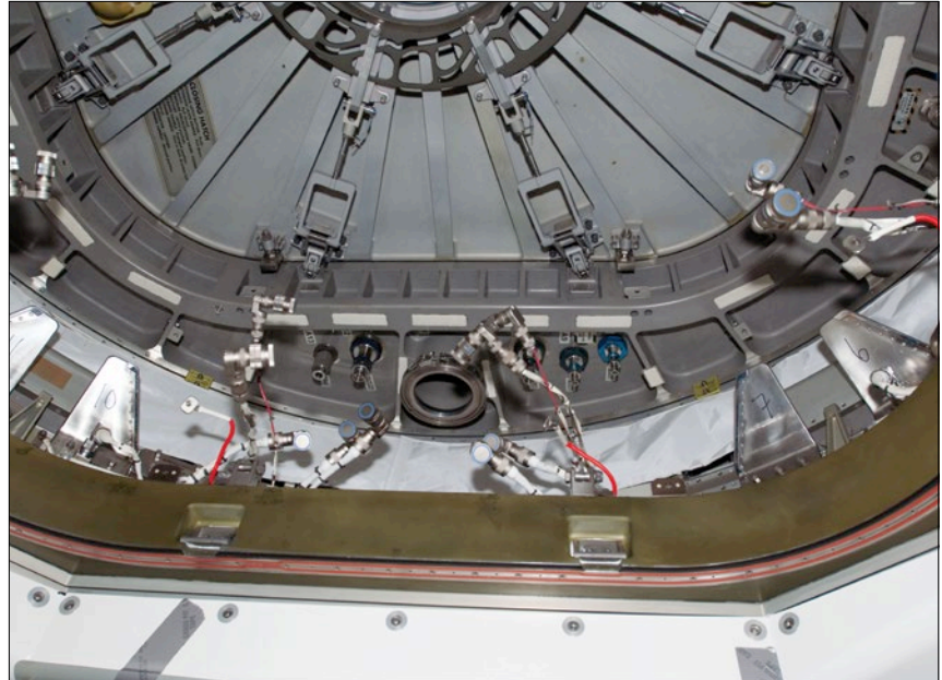
Figure 8. An example of a vestibule. This is the vestibule between Node 1 and Node 3 on STS-130/ISS-20A (2010) before all the power, data, and fluid jumpers were connected. Power and data cables for the active CBM are still installed (seen floating) but no jumpers are connected yet to the large or small feedthroughs on Node 3 (the module with the closed hatch).
