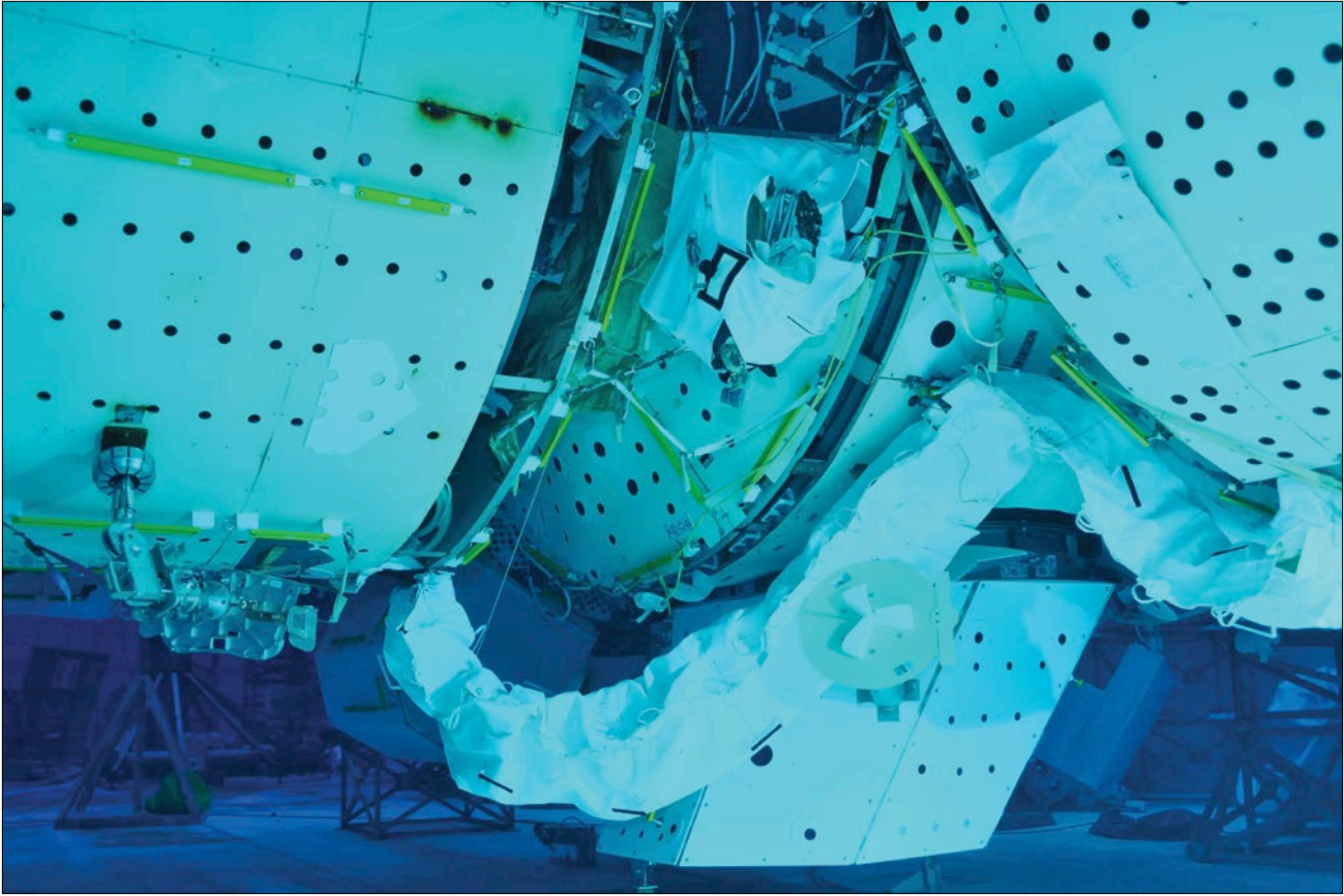
Figure 13. The billowy white insulation surrounding the ammonia lines at the NBL mock-up. This insulation drove the decision earlier on how to move PMA3 so as to not interfere with the PMM. Note that when the bag that held the ammonia lines was opened in the pool, the lines would shoot out toward the bottom like a crazed jack-in-the-box due to the orientation of the mock-ups in the water. Due to the problems with ammonia lines, as described, the final flight units were not ready for the mission until a few days before the mission. The spacewalking crew members wanted to handle the final items so they would have an idea as to what to expect on orbit. Therefore, the final days before the launch, they flew to Huntsville, Alabama, where the lines were being manufactured. Not only did they handle the ammonia jumpers, they packed the specially designed bag. The packed hoses were then rushed to the launch pad and stored in the orbiter. The crew members flew back to their quarantine facility at Kennedy Space Center.
