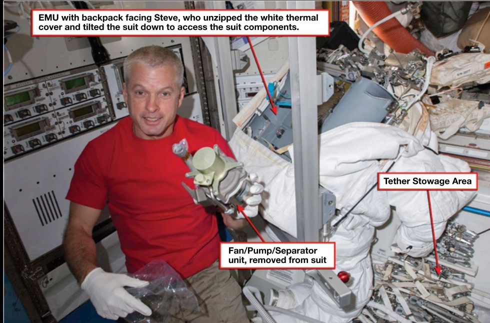
Figure 11. Astronaut Steve Swanson holds a Fan/Pump/Separator unit (with protective cylinder installed on the end). Several of these units were changed out in the on-board suits due to failures, as well as to investigate the cause of an incident on US EVA 23 where water entered a crew member's helmet. The EMU is installed in a rack that assists with suit donning, and it is tilted down with the backpack cover unzipped to expose the suit's life support system. Below the EMU is the tether stowage area in the Equipment Lock.
