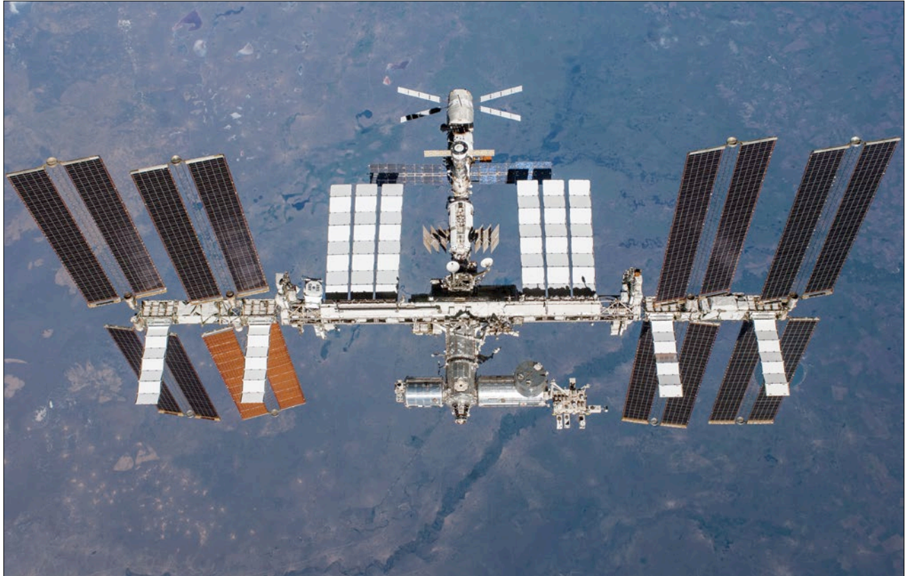
A picture of the International Space Station (ISS) showing the largest and most visible portions of the Thermal Control System: the radiator panels. Four white radiators project down in the photo, and provide dedicated cooling to the ISS Electrical Power System. Two sets of three larger radiators project upward in the image, and provide cooling to all the other systems on the ISS. Fluid lines loop through ISS systems, and the coolant within collects heat from computers, electronics, air conditioners, and other mechanical systems around the ISS. That heated coolant then flows through the radiators where the heat is rejected into space, and the coolant, returned to its starting temperature, runs through the same cycle again.
