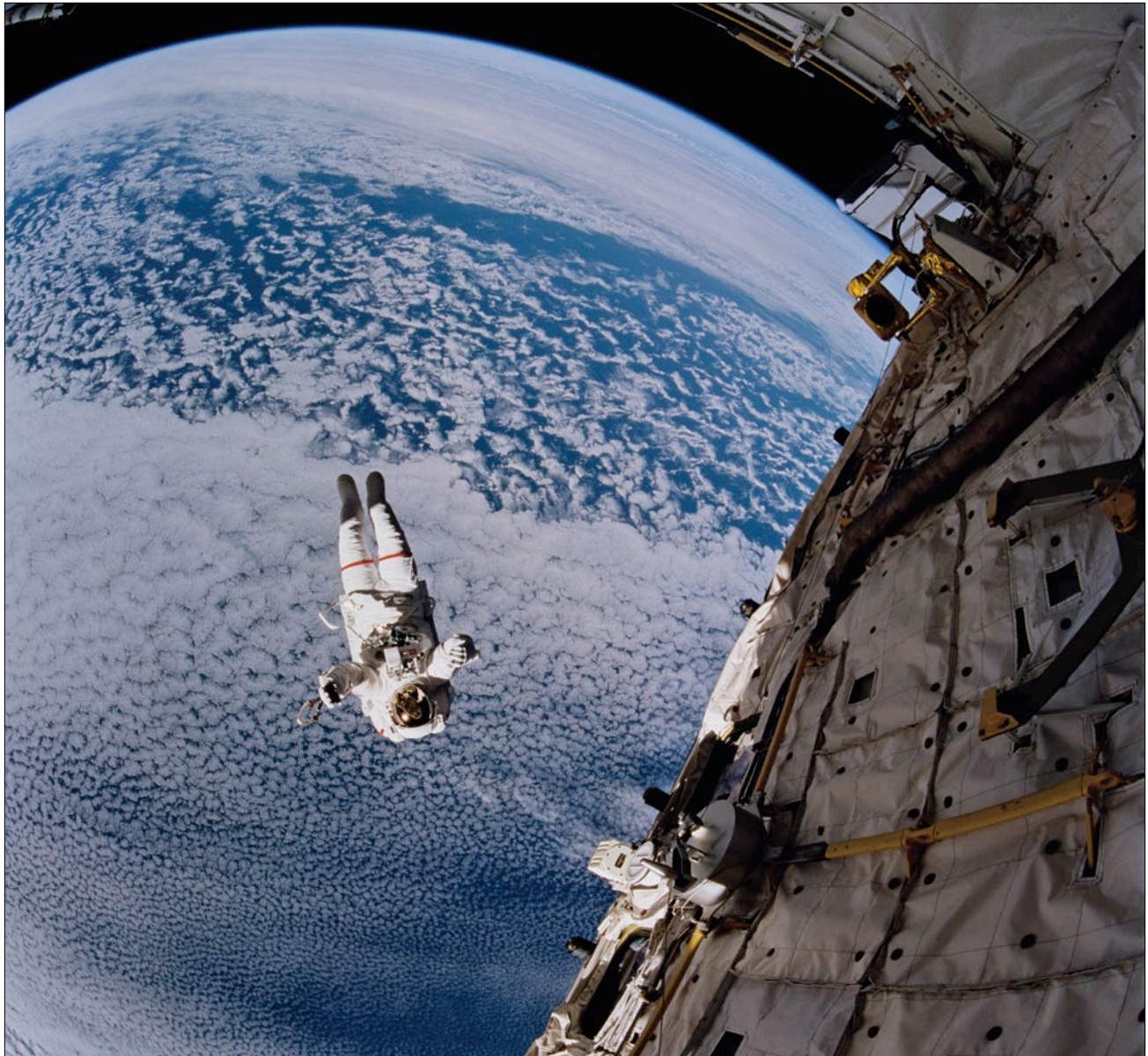
Figure 2. Astronaut Mark Lee tests the nitrogen-propelled backpack that would be needed for the ISS. Space Shuttle mission STS-64 (September 1994).
