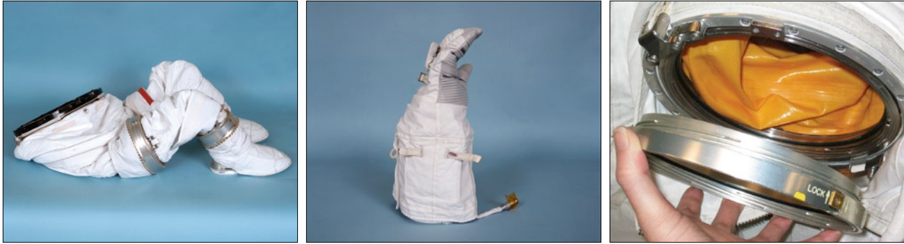
Figure 9. EMU components are specifically picked out for each crew member so the suit can be appropriately sized. Shown are: (left) the Lower Torso Assembly, with boots and metal sizing rings pictured; (center) an EMU glove; and (right) a sizing ring for lengthening an arm.
