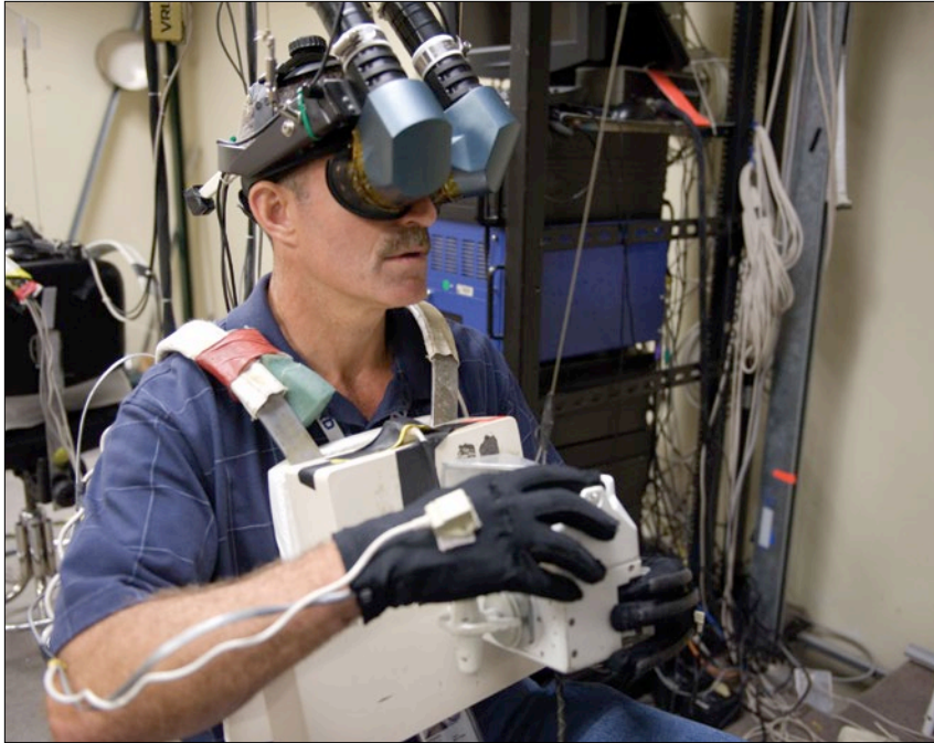
Figure 16. Astronaut Dan Burbank flies a mocked-up SAFER unit in the Virtual Reality laboratory. He is seeing the space station in 3-D and using the hand controller to “fly” back to the ISS. This provides a simulation of what it would be like if his tether broke and he detached from the structure.
