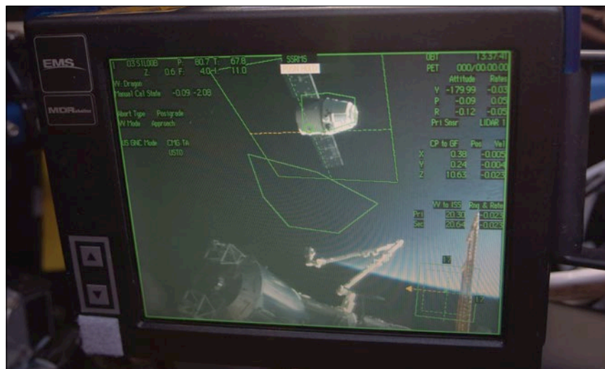
Figure 8. An example of using graphics overlay to capture a visiting vehicle—in this case, the first SpaceX Dragon spacecraft to the ISS. This picture shows one of the Robotic Workstation monitors during capture operations for the Dragon vehicle during Expedition 31 (May 25, 2012). The view of the ISS with the robotic arm and the incoming Dragon vehicle are provided by a camera mounted on the truss of the space station. The green lines, numbers, and letters define such things as a safe location for the spacecraft (e.g., the large green rectangle near top center) and the location where the vehicle is expected to be, as indicated by the green outline of the Dragon. These graphics are then overlaid on the video and shown to the crew member who is operating the arm. These overlays provide the crew member with real-time data about the Dragon, such as position and orientation, as well as outlining an imaginary approach corridor that the Dragon needs to maintain as it approaches the space station. Using overlays in this fashion allows the crew member to maintain situational awareness of the incoming vehicle without having to take his or her eyes off of the video showing the actual approaching vehicle.
