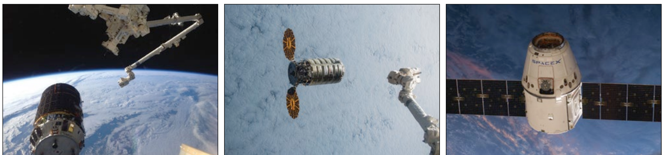
Figure 7. (Left) The robotic arm moves toward the unpiloted Japanese Kounotori HTV-4 as it approaches the ISS on August 9, 2013. The HTV-4 is delivering 3,600 kg (7936 lbs) of science experiments, equipment, and supplies to the orbiting complex. (Middle) Using the ISS robotic arm, seen at the right of the picture, NASA Flight Engineer Kjell Lindgren prepares to capture the Orbital ATK Cygnus cargo vehicle on December 9, 2015. The space station crew and the robotics officer in MCC-H will position Cygnus for installation to the orbiting laboratory’s Earth-facing port of the Node-1 module. (Right) The SpaceX Dragon Commercial Resupply Services-3 spacecraft approaches the ISS for rendezvous and grapple during Expedition 39 on April 20, 2014.
