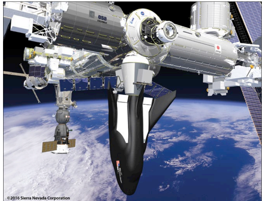
Figure 12. The Dream Chaser cargo vehicle, to be developed by Sierra Nevada Corporation, berthed to the nadir port of the Node 2 module. It is estimated to fly in 2020.
