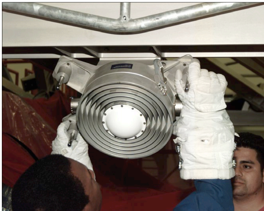
Figure 9. GPS antenna, one of four. The GPS antennas were designed to be replaceable by spacewalking astronauts. In this image, a technician fit checks an antenna while wearing spacesuit gloves to verify the design.
