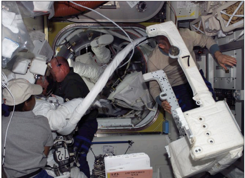
Figure 21. The SAFER on the right is attached to the EMU before the crew gets into the Crewlock for airlock depress. A hand controller, similar to a joystick, stays tucked into a storage area. If a crew member needs to rescue himself or herself by flying back to the ISS structure, the hand controller can be removed from storage quickly.
