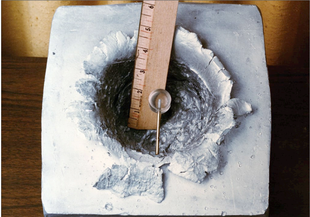
The potentially destructive nature of space debris. This photo (from a ground test) shows the damage done to a solid block of aluminum by a small 7-g (0.2-oz) projectile traveling at 7 km/s (4.3 miles/s).
